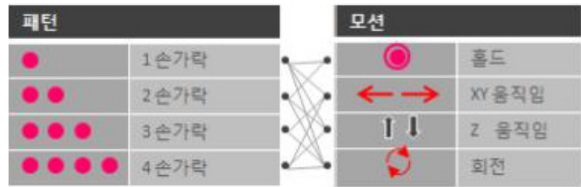
Figure 8 Finger Pattern and Motion for Gesture UX
