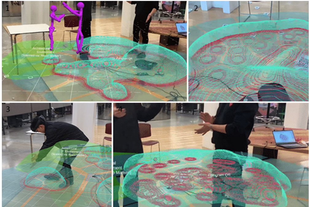
Figure 19 Multi-user simulations of a growth-regulated cell interface. (1) Users’ skeletal frames as they engage with the interface through body gestures and hand movements, (2) A close-up of the line-based fluid structure as seen through a HoloLens2 HMD, (3) A user experiencing the holographic interface overlaid in Mixed Reality, (4) A holographic interface responding to hand gestures, where proliferation rate, volumetric behavior of the metaball structure, and expansion levels are tied to the proximity values detected from the user’s moving hand skeleton. Reprinted from the first author’s master thesis “CELLNET: Bio-Inspired Adaptive Cellular Interface in Mixed Reality”, submitted to Cornell University, 2023
