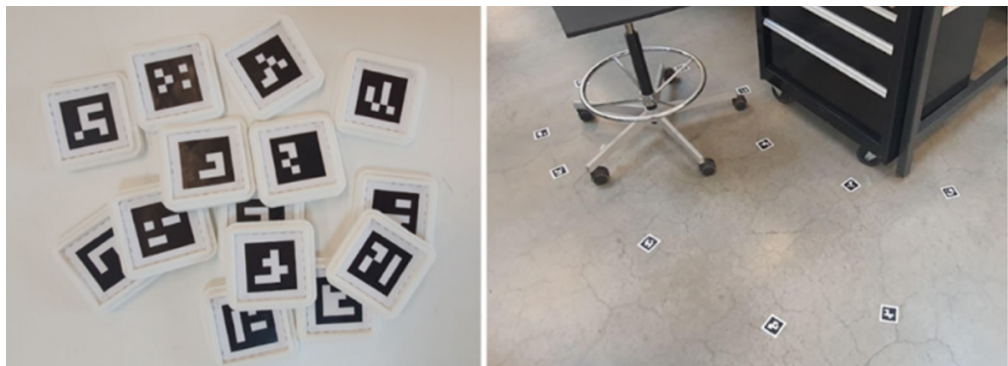
Figure 14 Aruco Marker pads used for mapping physical environments. To enhance stability, 3D-printed pads (15 mm thick) are attached to the markers before laying them out on the ground. Reprinted from the first author's master thesis "CELLNET: Bio-Inspired Adaptive Cellular Interface in Mixed Reality", submitted to Cornell University, 2023
