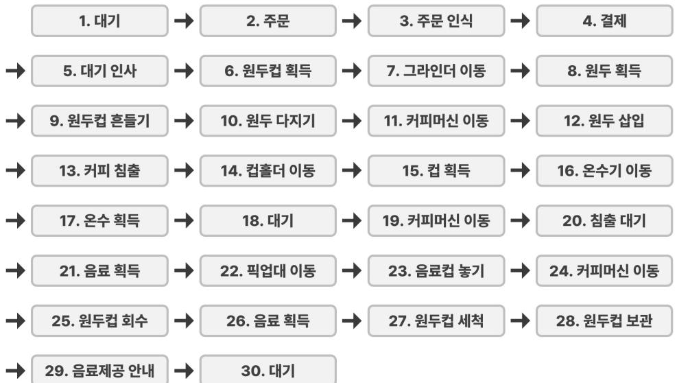
Figure 2 Coffee service process of cafe robo
