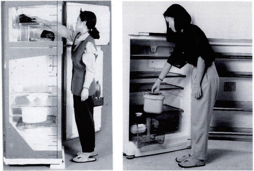
Figure 12, 13 Scenes from usability tests of refrigerator compartments (『산업디자인』, 1993)
