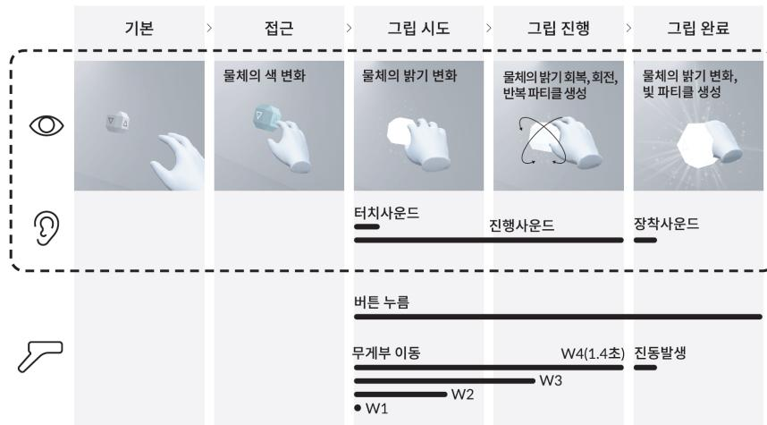
Figure 14 The audio-visual effects when holding an object
