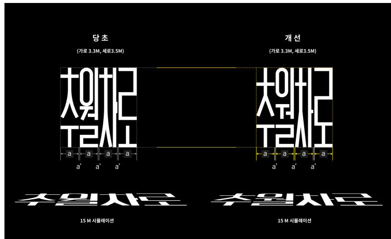
Figure 1 Pavement Marking Design Guide of Korea Expressway Corporation (Part)
