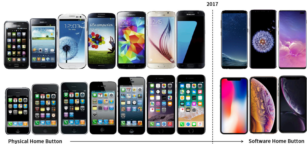
Figure 1 Home button transformation in the front of smart phone
