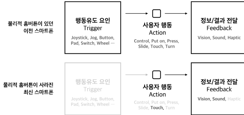
Figure 2 Interaction steps for previous and latest smart phone with and without physical home button in the front
