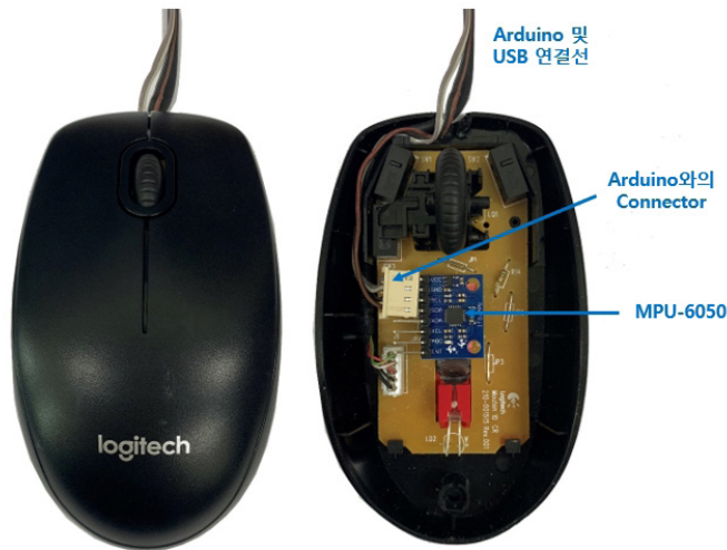
Figure 6 Installation of MPU-6050 sensor
