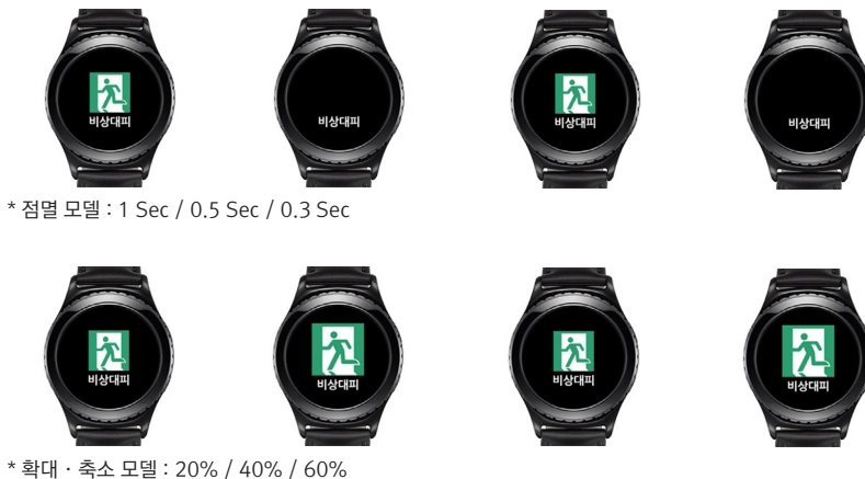
Figure 2 Motion variation in emergency evacuation model
