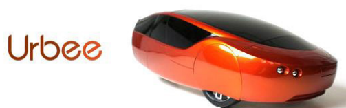
Figure 2 The 3D Printed Low-Energy Car 'Urbee' (Source: Chalcraft, E., 2013)
