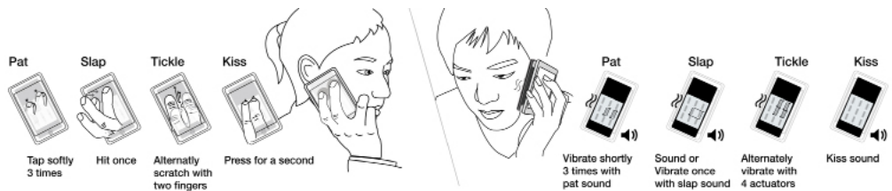
Figure 1 Representative examples to deliver pat, slap, tickle and kiss during phone conversations using vibrotactile stimulations and sound effect
