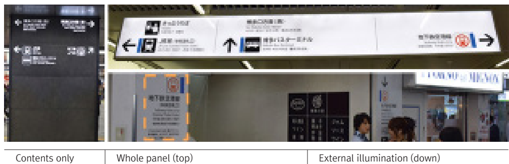
Figure 4 Illumination types of directional signs at the Station Concourse
