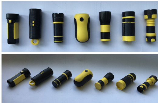
Figure 9 Models created using Rapid Prototyping
