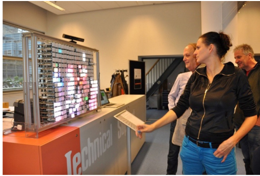
Figure 12 400 pixels assembled and with diffuser.
