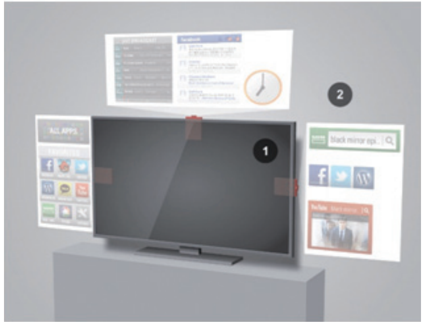
Figure 1 The two GUI layer of Beyond-screen interface: (1) foreground screen and (2) background screen (projected area)
