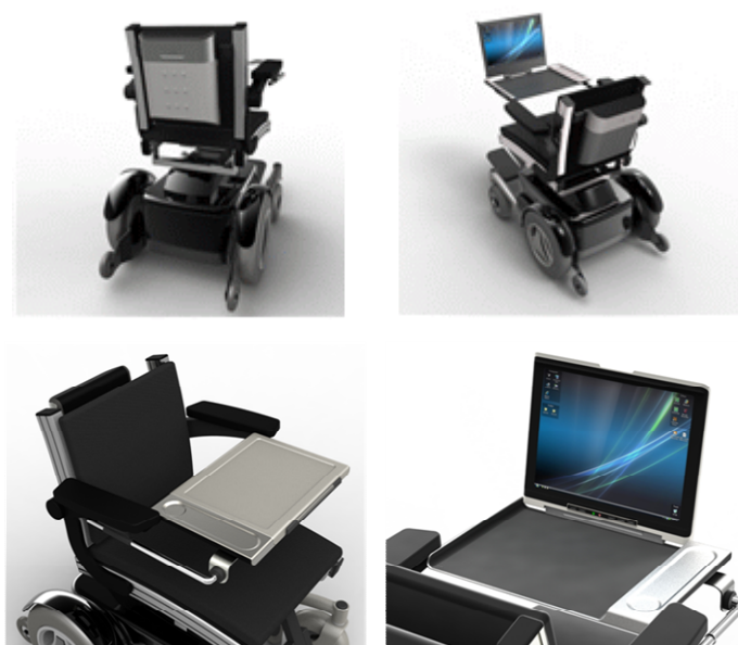
Figure 3. Design proposals of tray type computing system.
