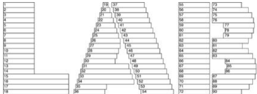
Figure 7 The final construction diagram of the LAB Logo. The height of each text frame is set to 12 pixels, considering the minimal type size for complex characters, such as Chinese
